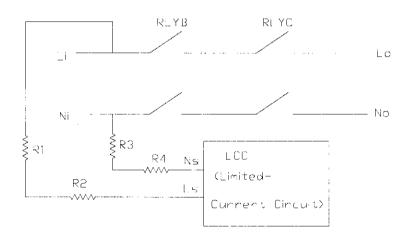
\* The air gap or sum of the air gap in each pole shall in accordance with Table 5 – Minimum clearance in secondary circuits and using the column headed "circuit not subject to transient overvoltage" for reinforced insulation at the working voltage that is backfed.
