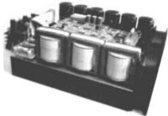
Fig.6: Photo of the prototype of the 10kW 2-U rectifier system. In front: Input choke in helical wound technology [12], right: 2 x 80mm high airflow fans, in the middle on top: control board realized in surface mount technology, in the back: output capacitors 6 x 330 \mu\text{F}/450\text{V} , in the left background: auxiliary power supply. Dimensions (without housekeeping, with fans): 230mm x 160mm x 88mm (2-U).
