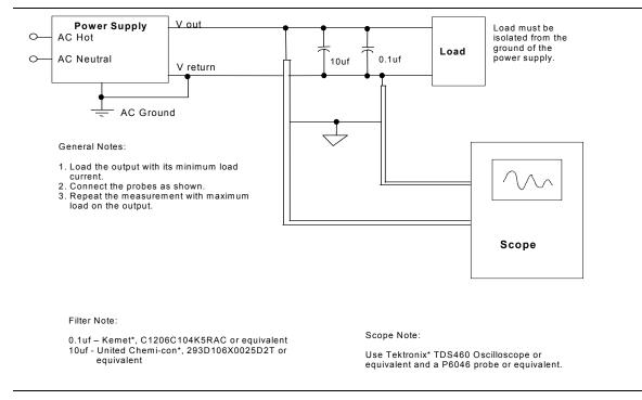
Figure 4. Differential Noise Test Setup
