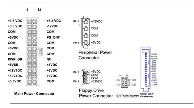
Figure 9. Connectors (Pin-side view, not to scale)
