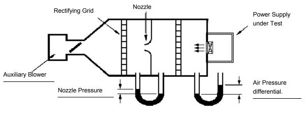
Auxiliary Blower is controlled to generate a zero Air Pressure differential. Air Flow is determined from Nozzle pressure.
