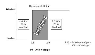
Figure 6. PS\_ON# Signal Characteristics
