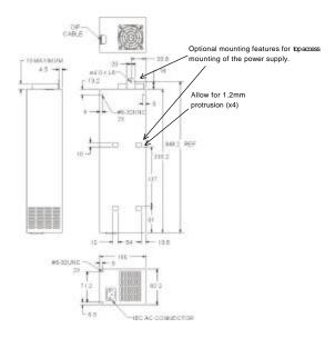
Figure 1: Enclosure Drawing
