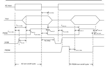
Figure 4: Turn On/Off Timing (Single Power Supply)
