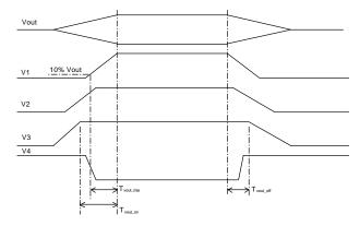
Figure 3: Output Voltage Timing
