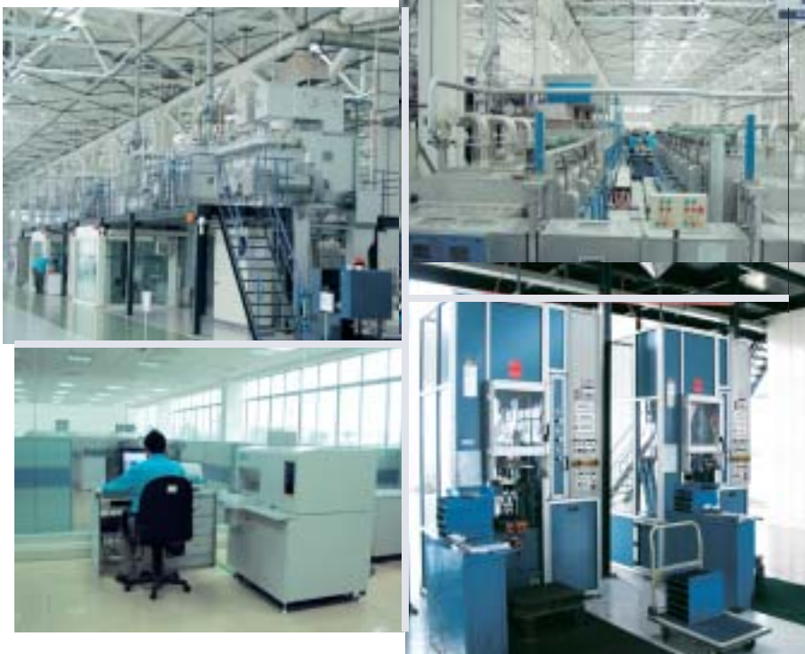
44米氮气保护隧道双轨窑 44m Double rail with N 2 auto-protection tunnel kiln
