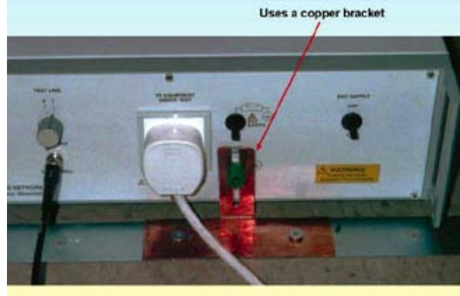
Figure 8 Example of good LISN GRP bonding
