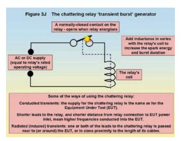
The chattering relay can be used in a wide variety of ways to generate radiated and/or conducted disturbances. If it is supplied via a safety-isolating transformer (or from a floating DC supply) with sufficient voltage withstand, the bottom side of the coil could be connected to the reference plane (or to any other conductor) and the top of the coil (the node that connects to the relay contact) could be connected via a
