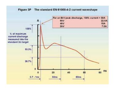
Figure 3P shows the standard waveform for the EN 61000-4-2 ESD test, which is a single unidirectional impulse. Figure 3R shows the basic scheme of an ESD generator or 'gun' and Figure 3S shows the standard bench test set-up. These three figures have all been developed from the EN 61000-4-2 standard.
