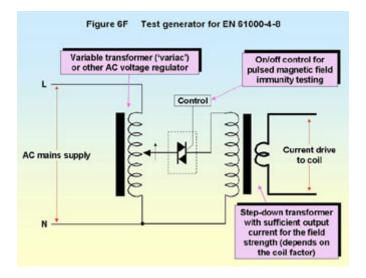
Driving a single-turn induction coil at 100A does not require very much voltage, so the secondary voltage for the step-down transformer might be as low as 3V rms. Induction coils with multiple turns will need proportionally less current for a given field strength, but will need a higher voltage drive.
