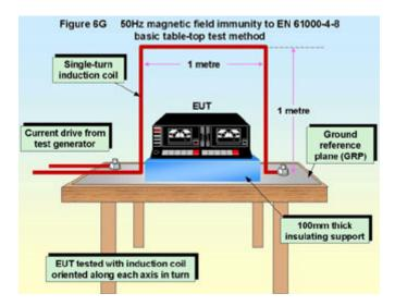
Apart from the test generator and induction coil(s) the test instrumentation required is some
