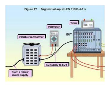
The test conditions are exactly the same as for dips and interruptions testing described in 6.5.1 above.
