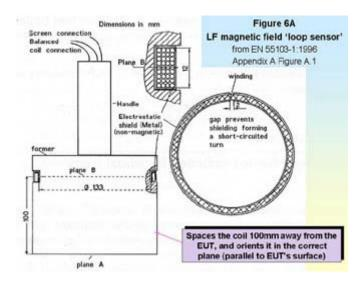
Calibration of the loop sensor is not necessary when it is constructed according to Figure 6A and the above conversion factor is used.
