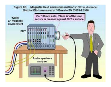
The loop sensor should be held at each test location for at least one sweep of the spectrum analyser. Where emissions could vary (for instance for an EUT that goes through a sequence of operations or states) many sweeps should be taken over at least one complete cycle of operation, preferably several, using the peak-hold mode of the analyser if one exists, so that the maximum readings are identified across the whole frequency range.
