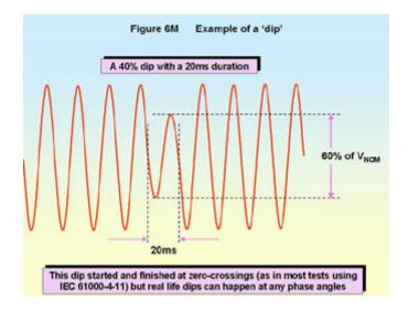
Dips may not occur in isolation - sometimes a fast sequence of dips occurs. Most immunity tests apply dips abruptly, starting and finishing at a zero crossing, but in practice they can have gentler rates of change and start and stop at any point in the mains cycle.
