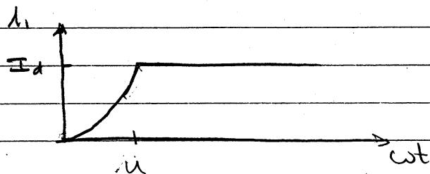
commutation ends at  $\omega t = u$  when  $I_1 = I_d$
