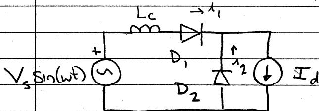
Assume we start with  $D_2$  conducting,  $D_1$  off ( $V_{sink} < 0$ )
