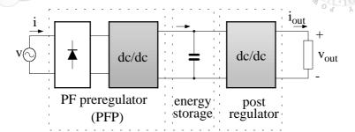
PREREGULATORS: AC/DC converters with high power factor and poor output voltage regulation
