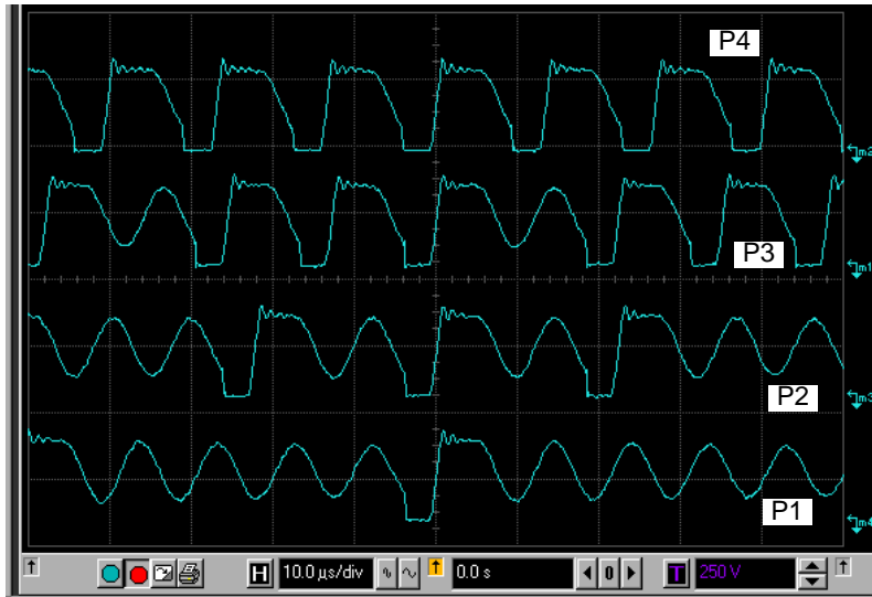
Figure 22. Drain-source signals at different powers: P1 < P2 < P3 < P4, you can note the multiple valley jumping.
