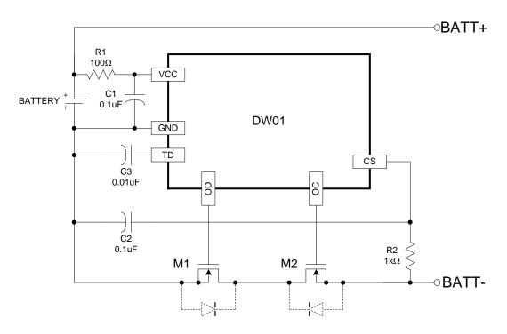
**Protection Circuit for One-Cell Lithium-Ion Battery**
