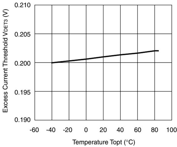
4) Short Circuit Protector Threshold vs. Temperature
