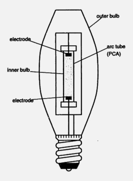
Figure 3-3: High pressure sodium lamp
