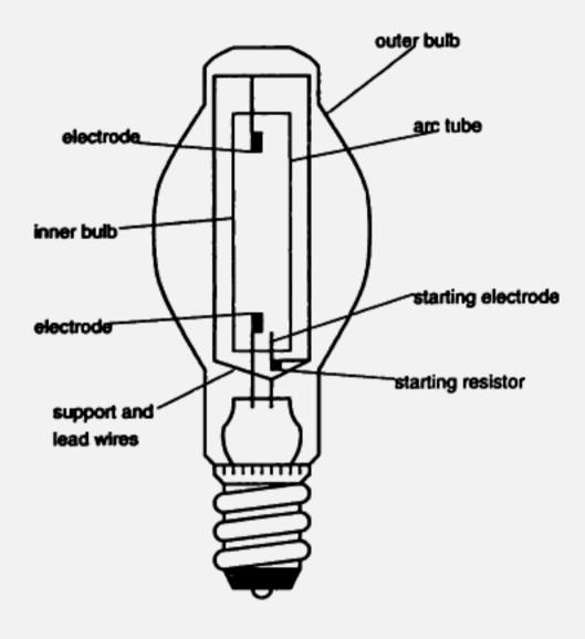
Figure 3-1: High pressure mercury vapor lamp
