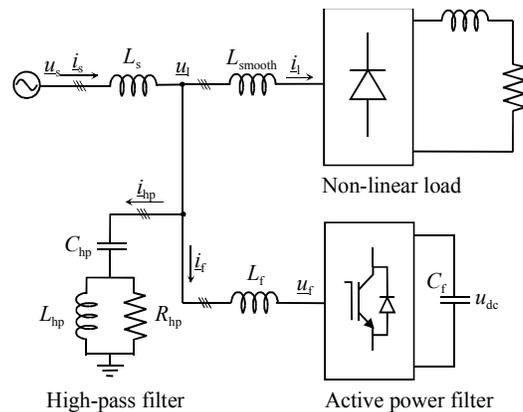
Figure 2. Configuration of the hybrid filter
