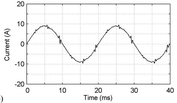
Figure 8. Measured phase-a supply current waveforms in the case of RC load current presented in Fig. 7 using a) the shunt APF with the control delay compensation method. b) the proposed method.
