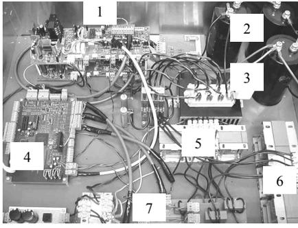
Figure 4. Prototype. 1 drivers, 2 dc link capacitors, 3 IGBT bridge, 4 microcontroller, 5 supply filter  $L_s$ , 6 filter inductor  $L_f$ , 7 current measuring
