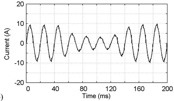
Figure 10. Measured phase-a current waveforms using the proposed method in the case of step change in the RC load. a) Load current. b) Supply current
