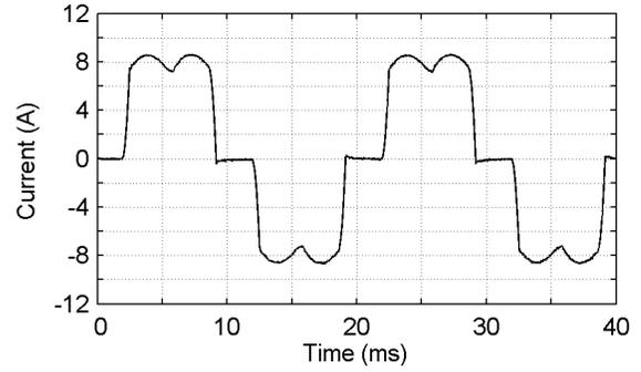
Figure 5. Measured phase-a load current waveform, using a three phase diode bridge supplying an RL load.
