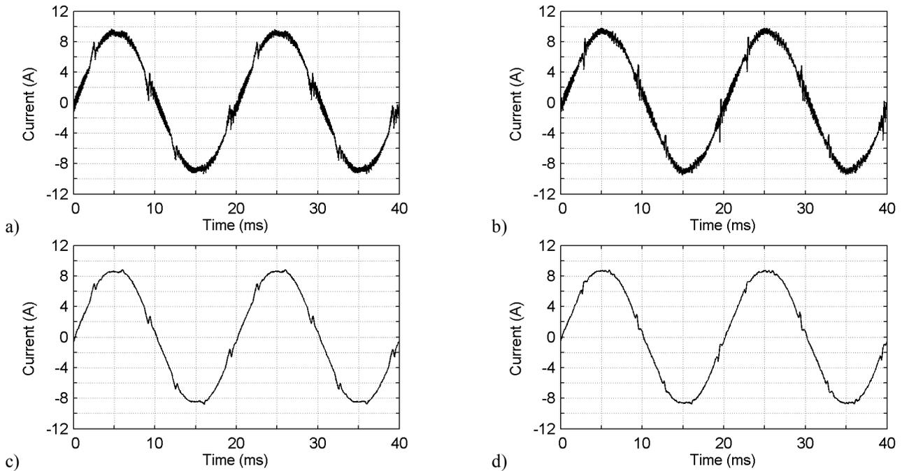
Figure 6. Measured phase-a supply current waveforms in the case of the RL load current presented in Fig. 5, using a) the shunt APF with a conventional control system b) the shunt APF with the control delay compensation method c) the shunt APF with the HPF and d) the proposed method.
