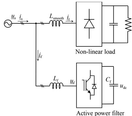
Figure 1. Configuration of the shunt APF
