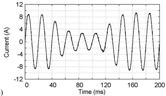
Figure 9. Measured phase-a current waveforms using the proposed method in the case of step change in the RL load. a) Load current. b) Supply current.
