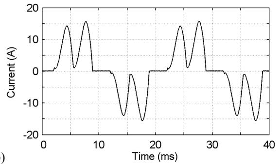
Figure 7. Measured phase-a load current waveforms, using a three phase diode bridge supplying an RC load. a) Shunt APF in operation. b) Hybrid filter in operation
