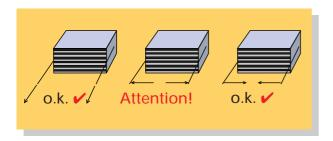
block of the ordering code). A torsional bending towards the centre of the capacitor is as uncritical as the axial stress mentioned above.
