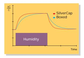
An unlimited contact of the SilverCap capacitor with water may destroy the contact between the metallization and the Schoop area and thus destroy the capacitor. For this reason wet surroundings must be avoided strictly. The microclimate, defined by IEC 721-3-9 in the interior of any electrical apparatus, must be according to these constraints in order to guarantee a successful application of the SilverCap capacitor.
