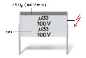
During the insertion of single-sided PC boards a direct contact of the Schoop areas to adjacent conducting parts and to the case has to be avoided. The minimum clearance as demanded by IEC 664-1 for peak voltages under 1000 V is 0.2 mm, which can easily be handled during hand insertion. We propose a minimum distance of  $\approx 1$  mm in order to take into account mechanical tolerances during the insertion of the PC boards.
