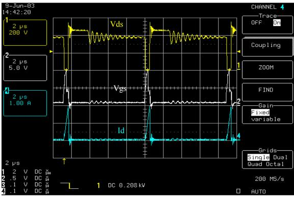
Normal Mode with 1A Load at Input Voltage 265V
