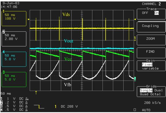
Burst Mode with No Load at Input Voltage 85V
