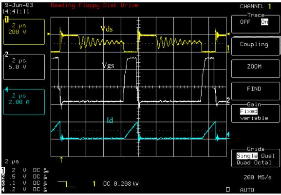
Normal Mode with 1A Load at Input Voltage 85V
