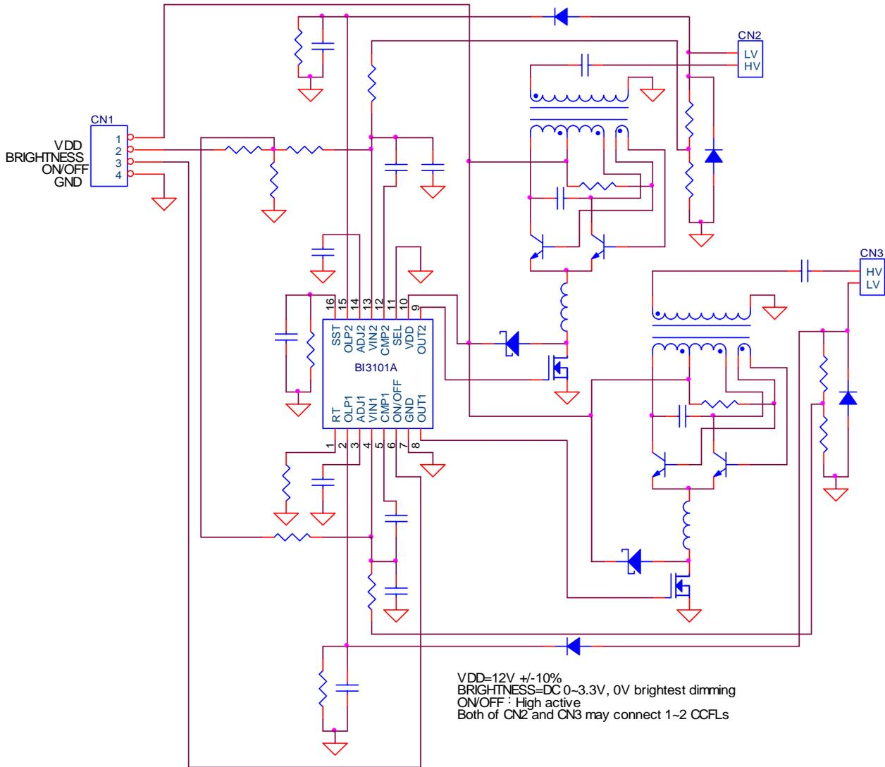
**Example2:** This is a different dimming scheme from Example 1, zero-volt-most-dark.
