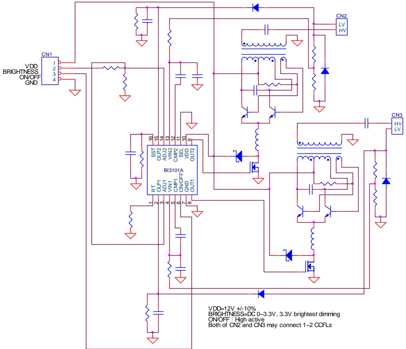
**Example3:** The independent design of open lamp protection makes BI3101A can used as a single PWM controller without consuming the extra power. A force-to-GND connection of OLP pin will shut down the circuit of PWM. This is an example of BI3101A operates as a single PWM modulator.
