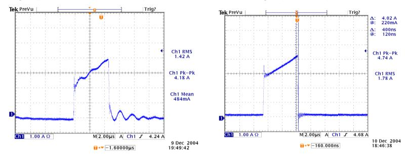
Sample C((before control run with OK A-core)) Ids開机30min后Ids波形仍OK: Sample D(with TDK core) Ids開机30min后Ids波形仍OK:
