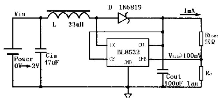
**(3) 测试保持电压电路 ( $I_{load}=1mA$ )**
