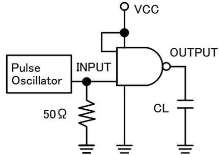
\* Output should be opened when measuring Current Consumption.
