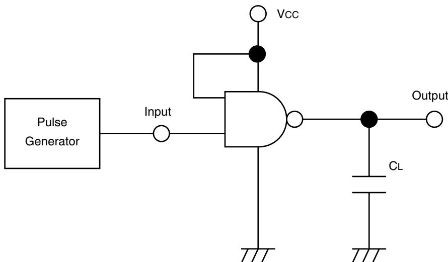
Note: open output when measuring supply current
