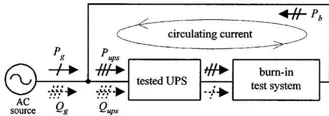
Fig. 1. Conventional UPS burn-in test system.
