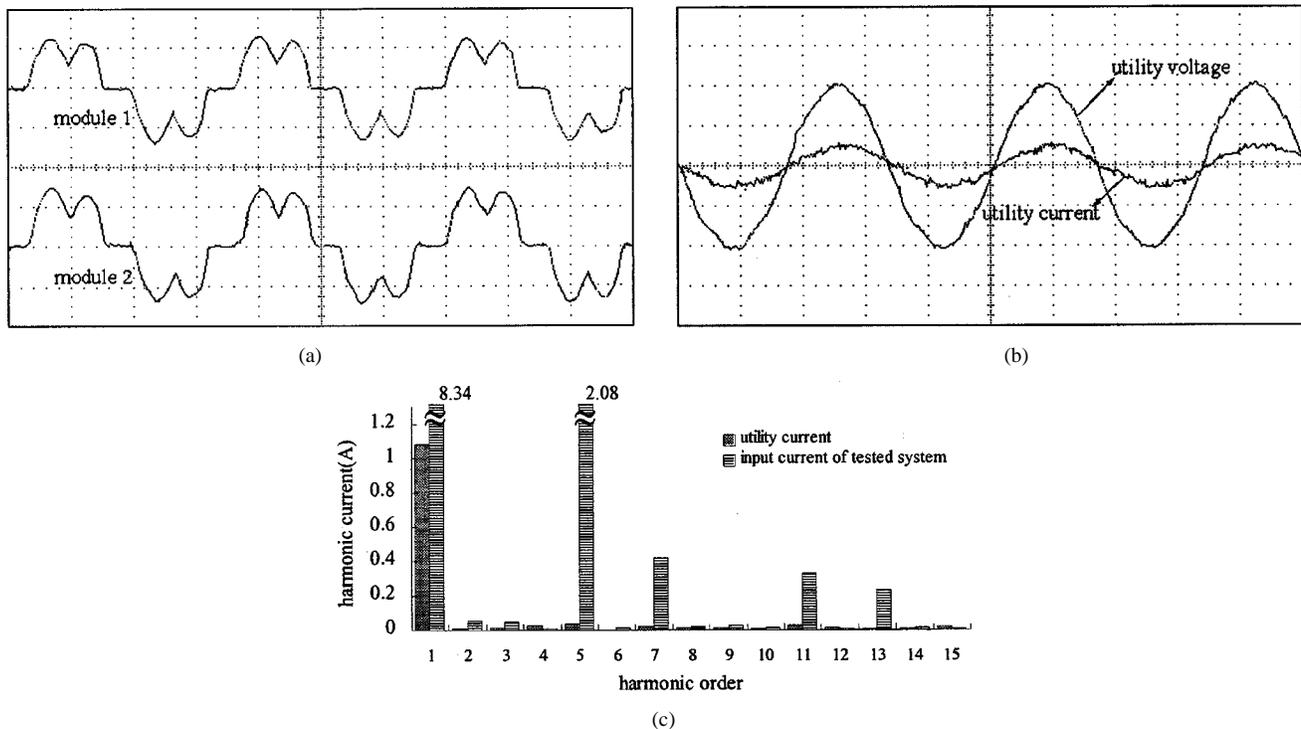
Fig. 10. Experimental results of burn-in test systems that are operated in parallel. (a) Input current of load module. (b) Utility voltage and current. (c) Spectrum of utility current and tested system input current.
