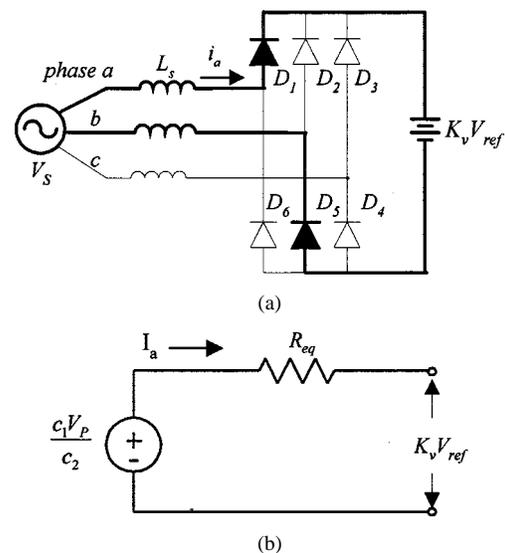
Fig. 3. Circuit model representing the circulating testing current control in the proposed system. (a) Circulating current flow. (b) Equivalent circuit.
