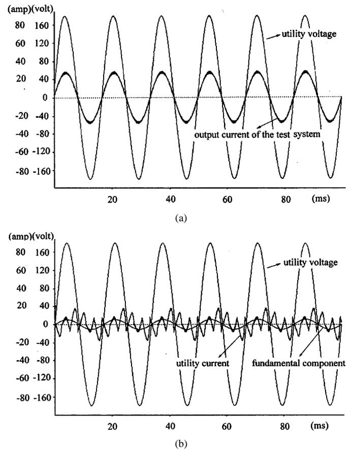
Fig. 7. Simulation results of the conventional burn-in test system. (a) Utility voltage and output current of the test system. (b) Utility voltage and utility current.
