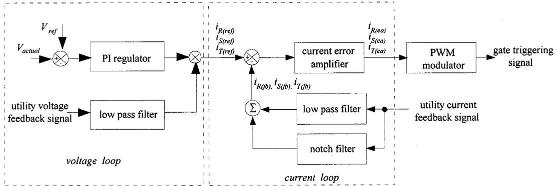
Fig. 4. Control block diagram of the inverter.
