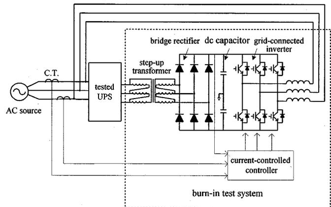
Fig. 2. Proposed burn-in test system.
