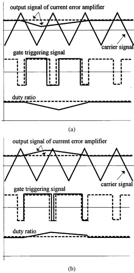
Fig. 5. Triggering signals generation in the controller when undesired noises appear. (a) Spike noise. (b) Dip noise.
