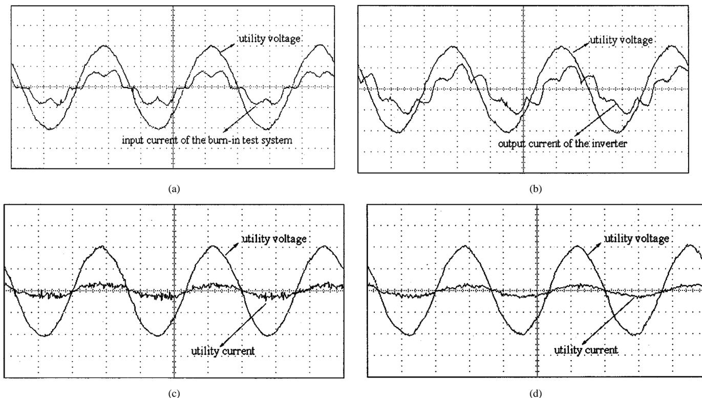
Fig. 8. Experimental results of the proposed burn-in test system. (a) Utility voltage and input current of the burn-in test system. (b) Utility voltage and output current of the inverter. (c) Notch filter is not included in the controller. (d) Notch filter is included in the controller.
