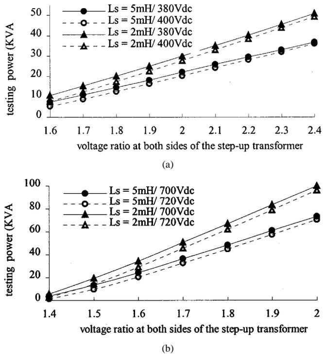
Fig. 6. Relationships between the testing capacity and dc capacitor voltage. (a) For 120/208-Vac system. (b) For 220/380-Vac system.
