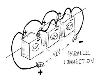
In case you need increased battery capacity or the possibility to connect heavy loads you can connect batteries in parallel. This means that you connect the positive terminal of one battery to the positive terminal of another battery. The voltage of this connection will still be that of one single battery but the capacity will be increased and the ability to handle heavier loads will increase.
