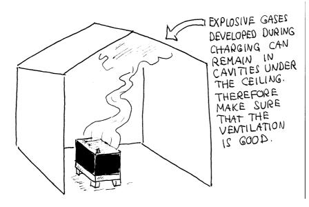
Most important is to facilitate ventilation of the battery room to prevent accumulation of explosive gases as well as acid mist.
