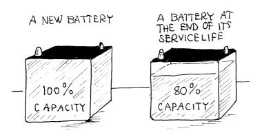
It is also important to understand that the nominal capacity relates to the capacity obtained from a new battery. The end of life is defined as the point where the capacity has declined to 80 % of the nominal value.
