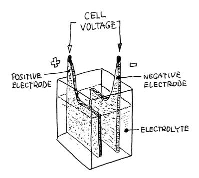
When a battery is connected to an external load a chemical reaction takes place between the electrodes through the electrolyte. The chemical energy converted is to electrical energy and current from positive the electrode through the load and back to the negative electrode.
