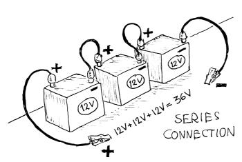
For some purposes one might need a higher voltage than that of a single battery. It is then possible to connect batteries in series. This means that you connect the negative terminal of one battery to the positive terminal of another battery.
