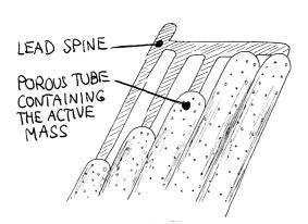
In tubular plates, where a lead spine is surrounded by a highly porous, plastic tube, the active mass is located between the lead spine and the tube. The high current capability of this type of electrode is nevertheless limited, since one cannot reduce the dimension of the tubes. The normal tube diameter is 8 mm (discharge time 3 - 10 h), which can be reduced to 6 mm for specific higher power applications (discharge time 1 - 3 h).
