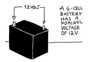
The voltage of a battery can be compared to the *height difference* in meters between the surface of a hydropower dam and the turbine outlet. (The current in Amperes can be compared to the water flow in m3 per second)
