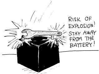
The short circuit current is normally very high, especially for a starter (SLI) battery. Severe accidents have been reported when a person has tried to remove the object creating the short. These objects are most often extremely hot and will create severe damage to the hands. The arc that will come when removing the tool may also start an explosion.
