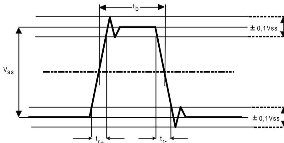
$V_{ss}$ =Voltage difference between steady-state signal conditions;
