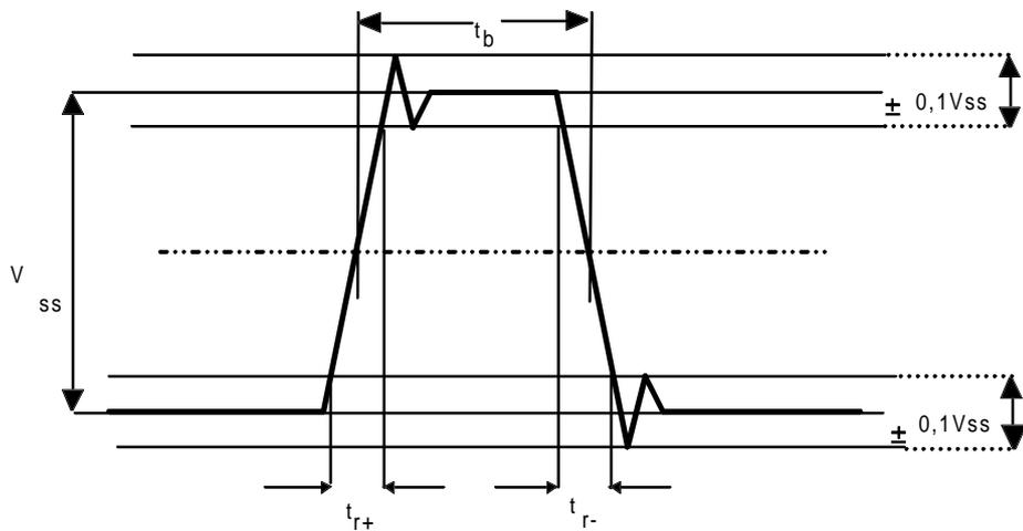
$V_{ss}$ =Voltage difference between steady-state signal conditions;
