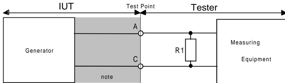
NOTE: The shaded area denotes an interconnection means e.g. Interface cable and connector.
