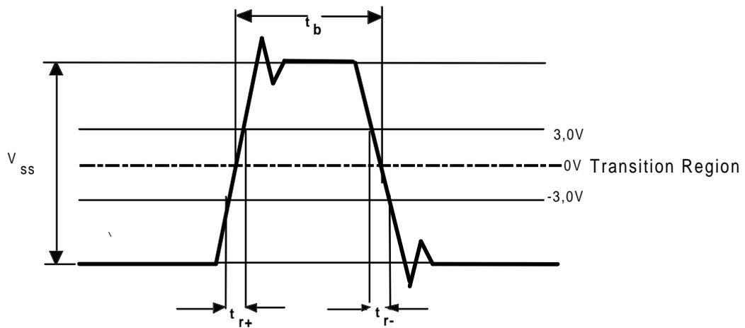
$V_{ss}$  = Voltage difference between steady-state signal conditions;
