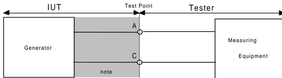
NOTE: The shaded area denotes an interconnection means e.g. interface cable and connector.
