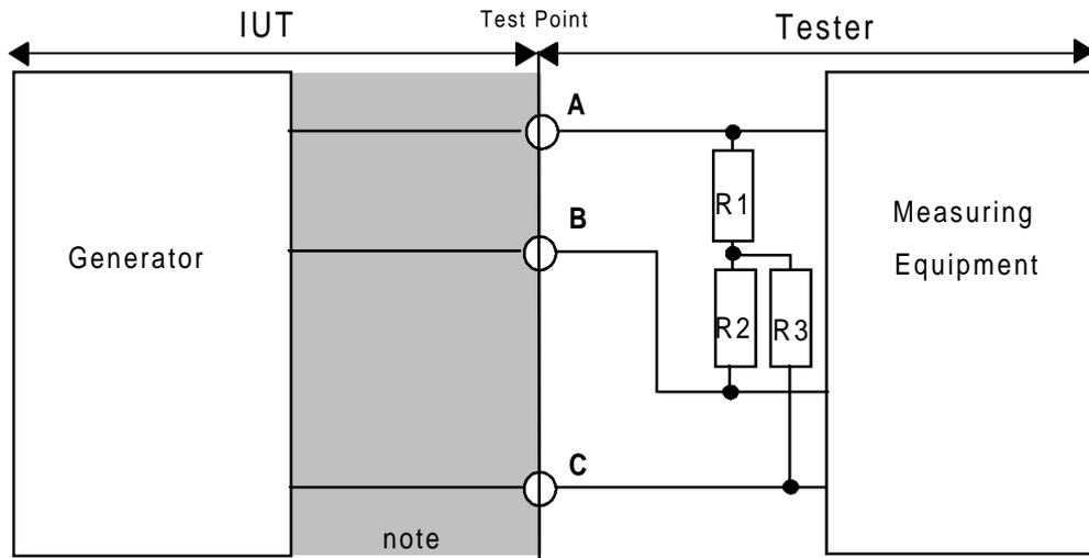
NOTE: The shaded area denotes an interconnection means e.g. interface cable and connector.
