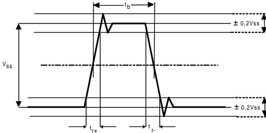
Vss=Voltage difference between steady-state signal conditions;
