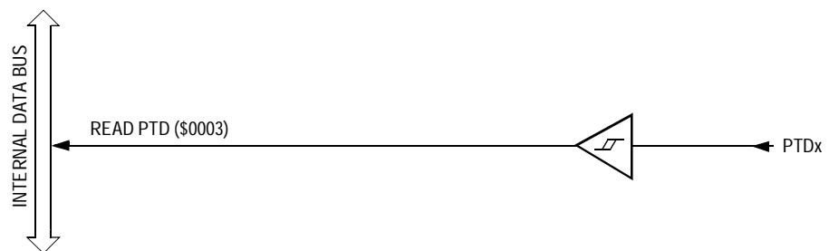
Figure 15-12. Port D Input Circuit
