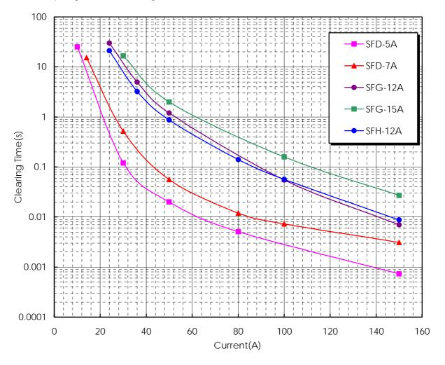
6.1. Current interrupting time (Ambient temperature vs. Clearing time by Rated Current \* 2)
