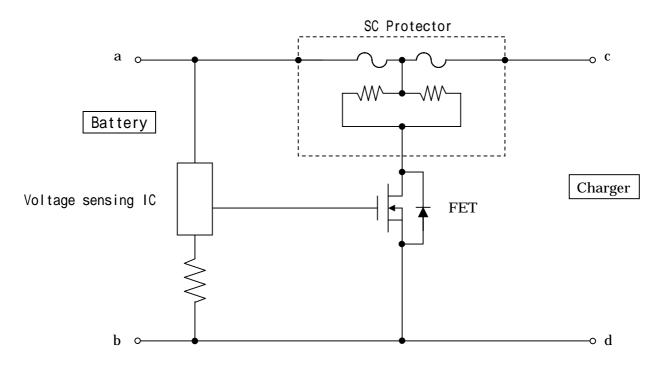
When the voltage between a and b exceeds the pre-set limit value, the output of the voltage detector IC becomes high and the FET is switched on. As a result, current flow through the heater of the protector, the fuses melt, and the battery stops to be charged any longer.
