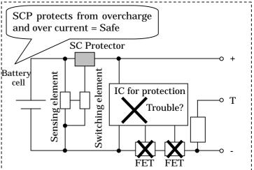
element forcibly fused by the heating of the heater and, upon the cutoff of charging circuit, the current to the heater automatically stops, and hence, SC Protector itself never overheated.
