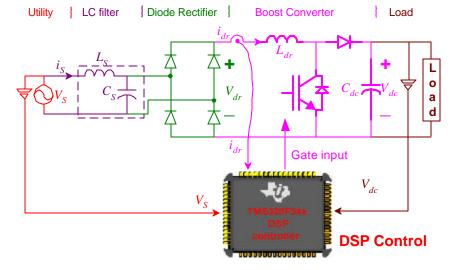
Fig. 2 Digital control of PFC Boost Converter.
