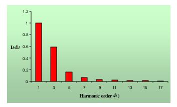
(c) Harmonics of diode rectifier current
