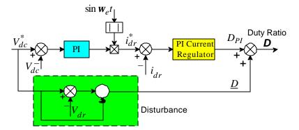
Fig. 4 Control block diagram for the proposed PFC boost converter.
