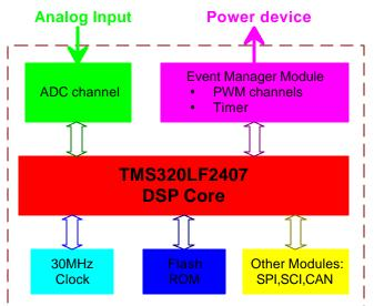
Fig. 6 TMS320LF2407 DSP simplified hardware diagram.
