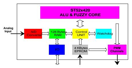
Fig. 8 ST-Fuzzy Studio (ST52x420) architectural block diagram.
