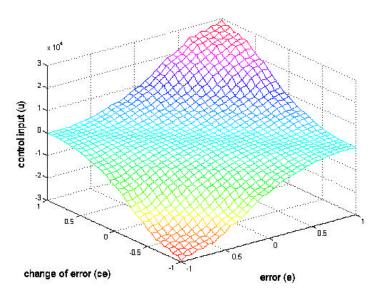
Fig. 7 The output of fuzzy logic controller obtained from off-line computation.
