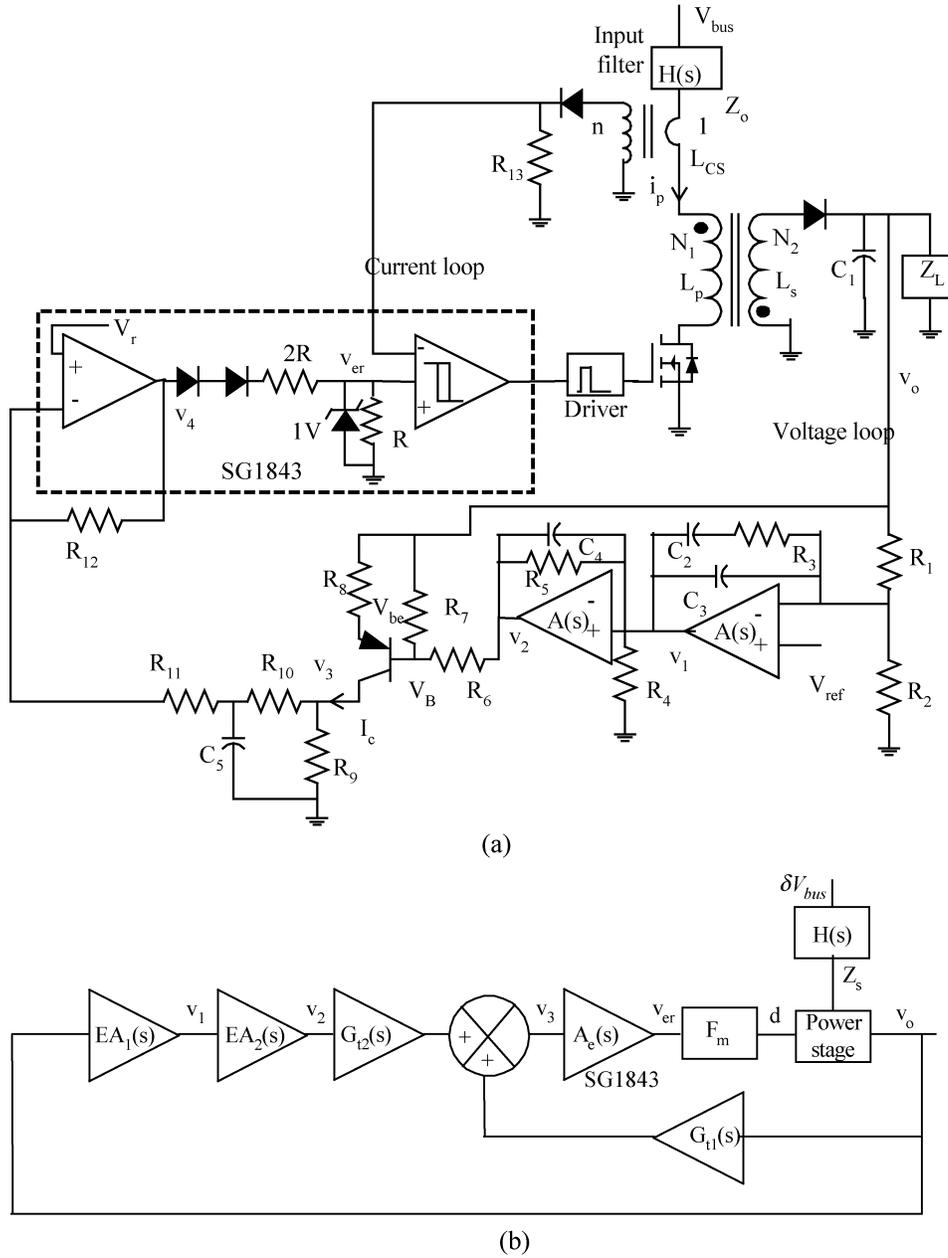
Fig. 1. (a) Circuit schematic. (b) Small-signal block diagram.
