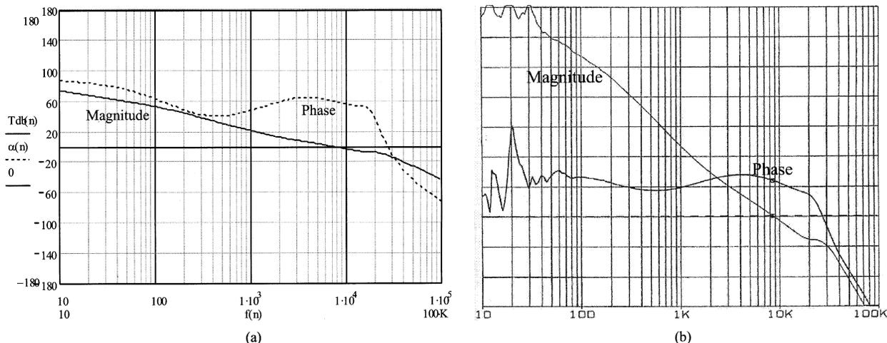
Fig. 2. Loop gain. (a) Theoretical. (b) Measurement 10 dB/div, 45°/div.
