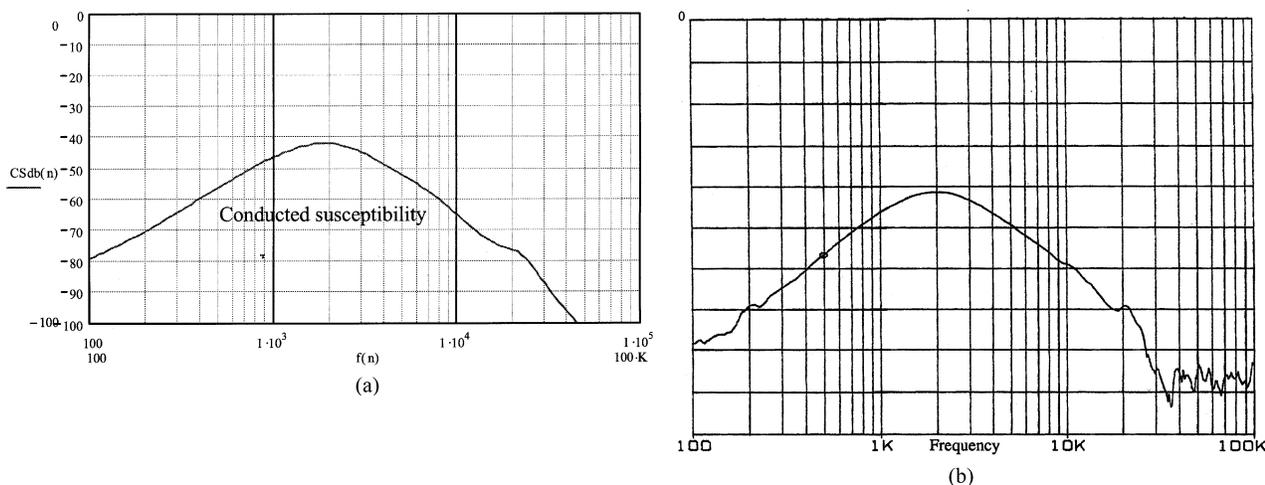
Fig. 3. Conducted susceptibility. (a) Theoretical. (b) Measurement. -10 dB/div.
