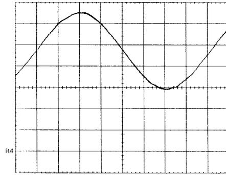
Fig. 17. Voltage across the capacitor  $C_1$  (50 V/div-2 ms/div).
