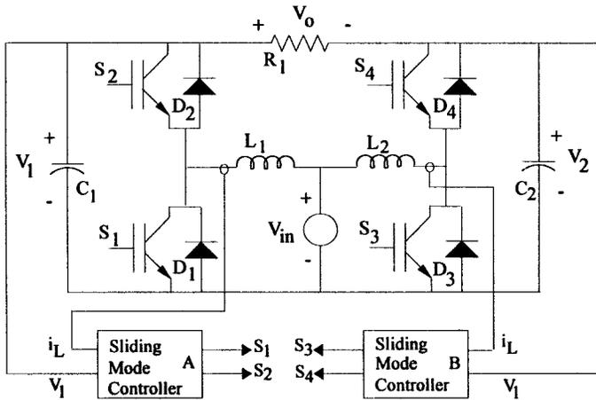
Fig. 7. The boost inverter controlled by sliding mode.
