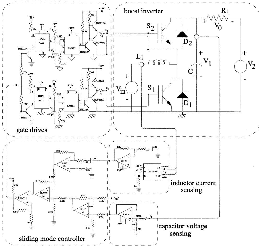
Fig. 13. Boost inverter scheme with sliding mode controller.
