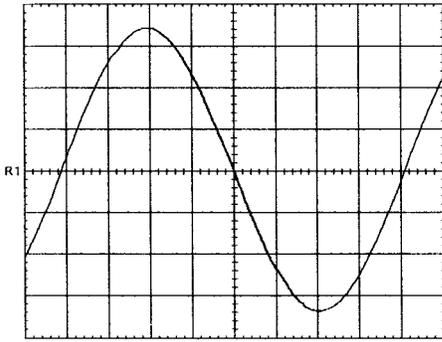
Fig. 14. Output voltage, nonload (50 V/div-2 ms/div).
