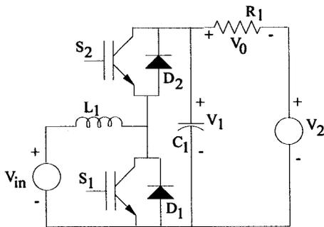
Fig. 8. Equivalent circuit for the boost inverter.
