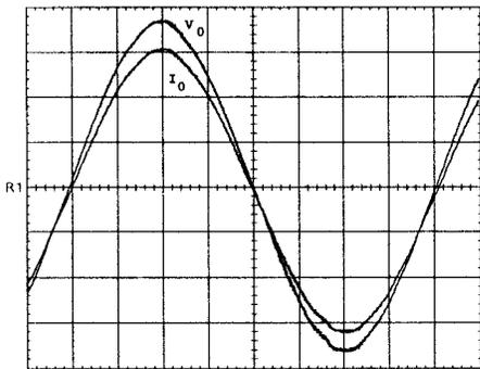
Fig. 15. Resistive load operation (50 V/div-2A/div-2 ms/div).
