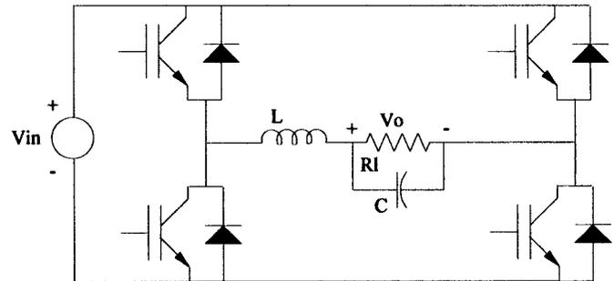
Fig. 1. The conventional VSI or buck inverter.
