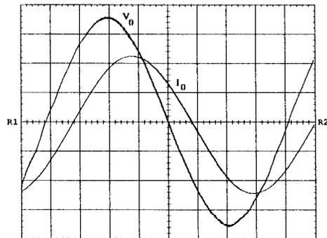
Fig. 18. Inductive load operation (50 V/div-2 A/div-2 ms/div).
