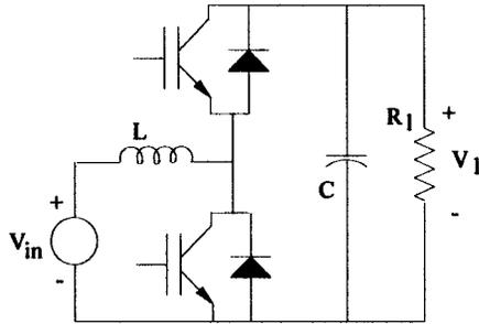
Fig. 4. The current bidirectional boost dc-dc converter.
