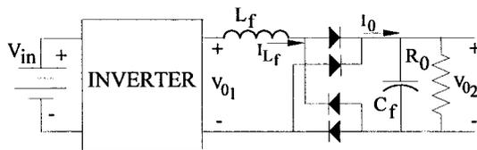
Fig. 19. Nonlinear load used with the boost inverter.
