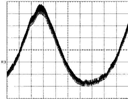
Fig. 16. Current through the inductor  $L_1$  (5 A/div-2 ms/div).
