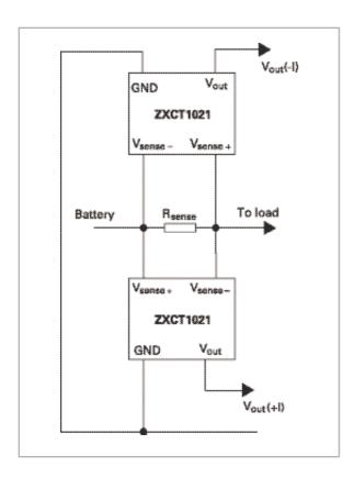
In applications such as battery monitoring, it is necessary to measure current flowing in two directions. This can be achieved with the ZXCT series by connecting 2 devices back to back, as shown in the applications drawing.
