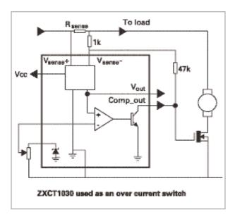
The on-chip comparator and reference provides functions commonly used for current and power control. By the addition of an N-channel switch and a few resistors it is possible to make an electronic fuse.
