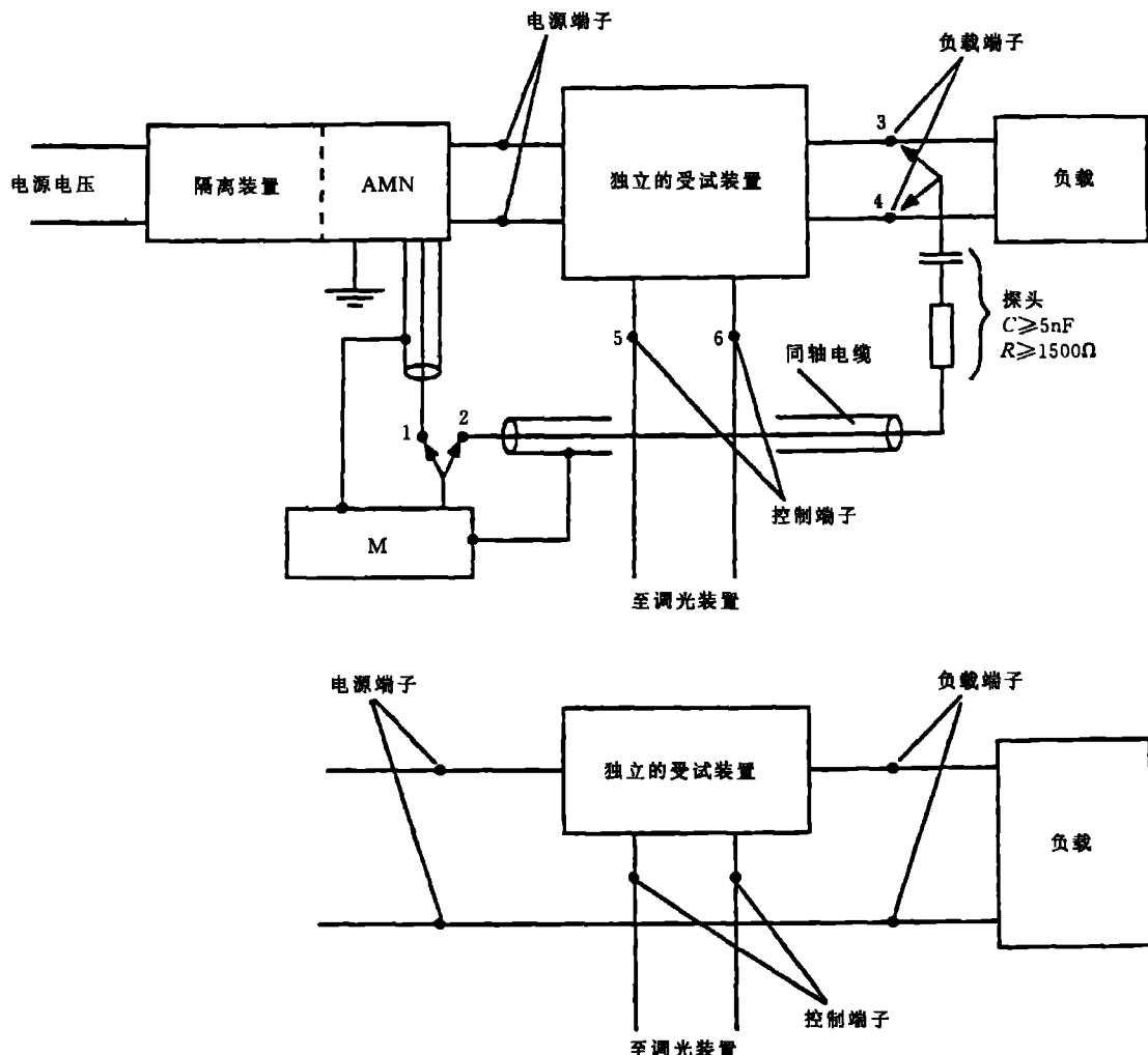
AMN - CISPR 16-1 规定的  $50 \Omega/50 \mu\text{H} + 5 \Omega$ (或  $50 \Omega/50 \mu\text{H}$ )人工电源网络
