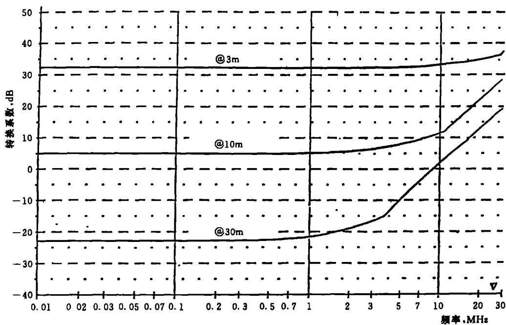
(电流  $\text{dB}\mu\text{A}$  + 转换系数(dB) = 磁场( $\text{dB}\mu\text{V/m}$ ))
