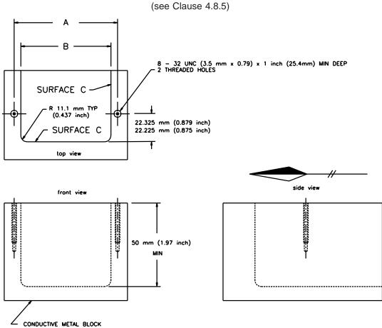
Figure 1 Test fixture for flush device clearance to flush-device box
