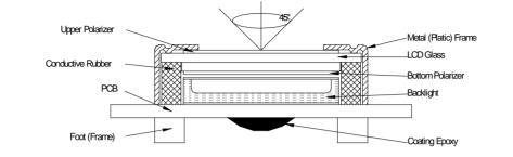
2. View Angle: with in 45° around perpendicular line.
