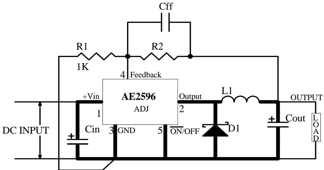
$$V_{OUT} = V_{REF} \left( 1 + \frac{R_2}{R_1} \right) \quad R_2 = R_1 \left( \frac{V_{OUT}}{V_{REF}} - 1 \right) \quad V_{REF} = 1.23V$$
