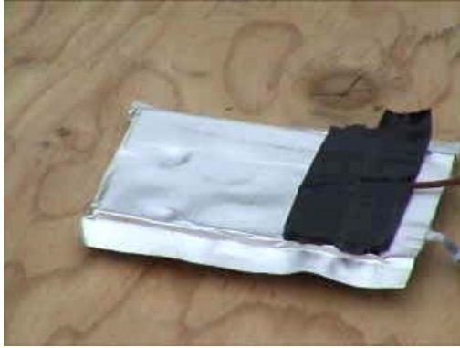
Figure 6. Photograph showing damage inflicted onto a lithium-ion gel-polymer cell by several hammer blows.
