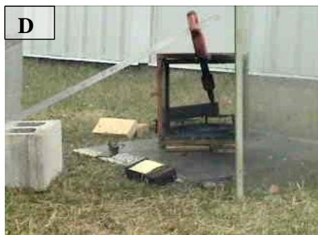
Figure 3. A. Photograph of a BA-521 battery; B. a lithium-thionyl chloride version of the battery in the nail test apparatus. C. the battery exploding (see text). D. the damaged apparatus.
