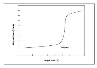
Protection is accomplished by limiting the current flow to some leakage level. Leakage current can range from less than a hundred milliamps at rated voltage up to a few hundred milliamps at lower voltages. The fuse on the other hand completely interrupts the current flow and this open circuit results in "0" leakage current when subjected to an overload.
