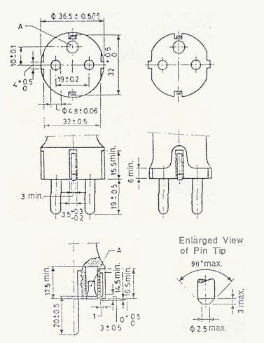
A: Flexible connection tube of 4.3~5.1mm (The shape may not necessarily be tube type)
