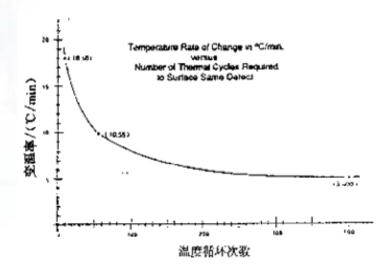
Temperature transition rate and the temperature cycle times of Stimulation failure relationship
