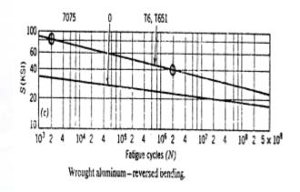
Al bending stress and failure cycle time relationship
