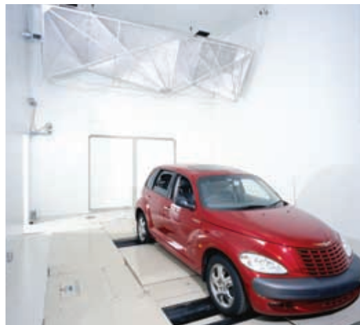
Fig. 1 Companies can use reverberation chambers to test large UUTs because they provide relatively large test volumes. Note the stirrer/tuner in the rear of the chamber.
