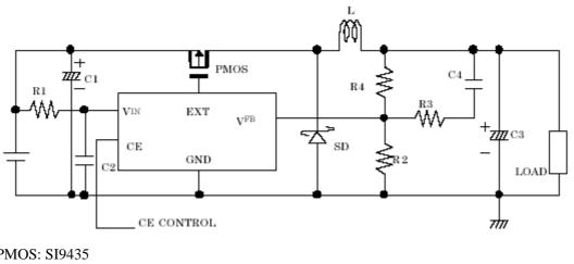
PMOS: SI9435 L: 27  $\mu$  H SD1: 1N5817 C1: 10  $\mu$  F (Ceramic Type or Electrolytic Type) C2: 0.1  $\mu$  F (Ceramic Type or Electrolytic Type) C3: 47  $\mu$  F (Caramic Type) C4: 1000pF (Ceramic Type) R1=10 $\Omega$ , R2=14.3k $\Omega$ , R3=2.7k $\Omega$ , R4=33k $\Omega$
