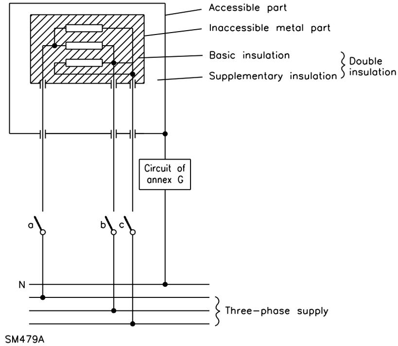
**Figure 7 – Diagram for leakage current measurement at operating temperature for three-phase connection of appliances other than those of CLASS II**
