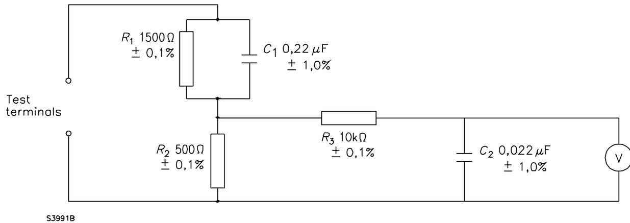
The leakage current is calculated from the reading of the voltmeter divided by 500  $\Omega$
