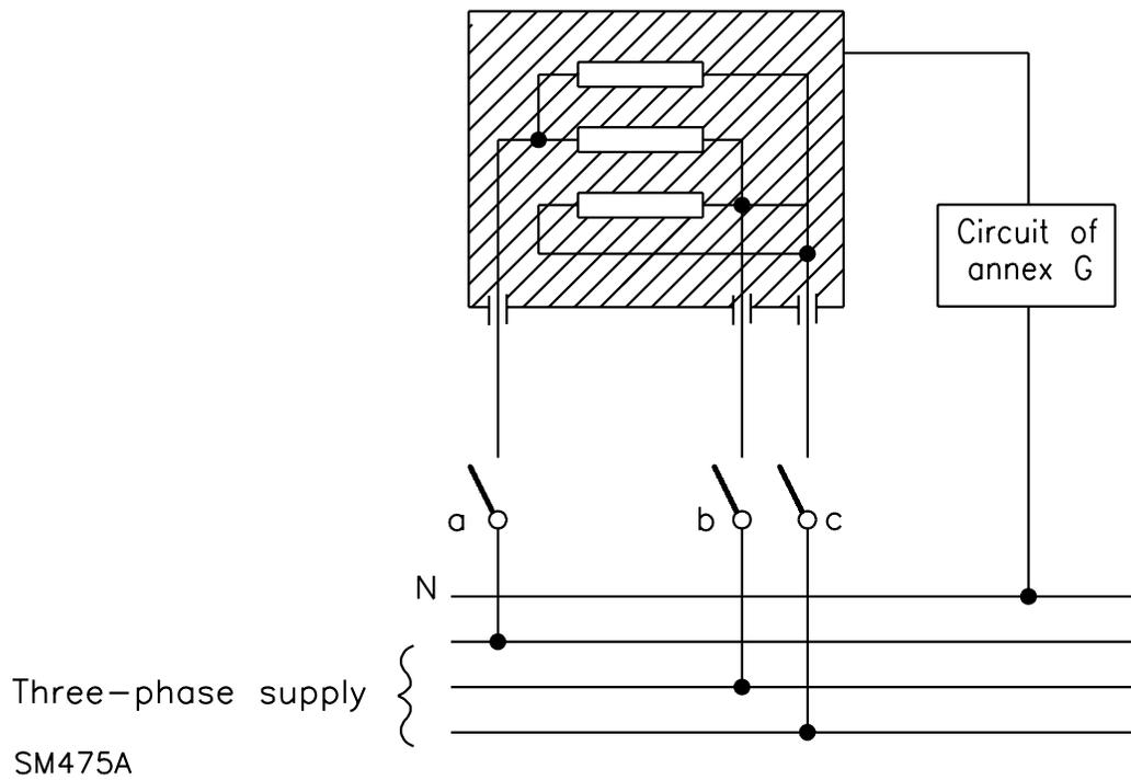
Figure 8 – Diagram for electric strength test at operating temperature
