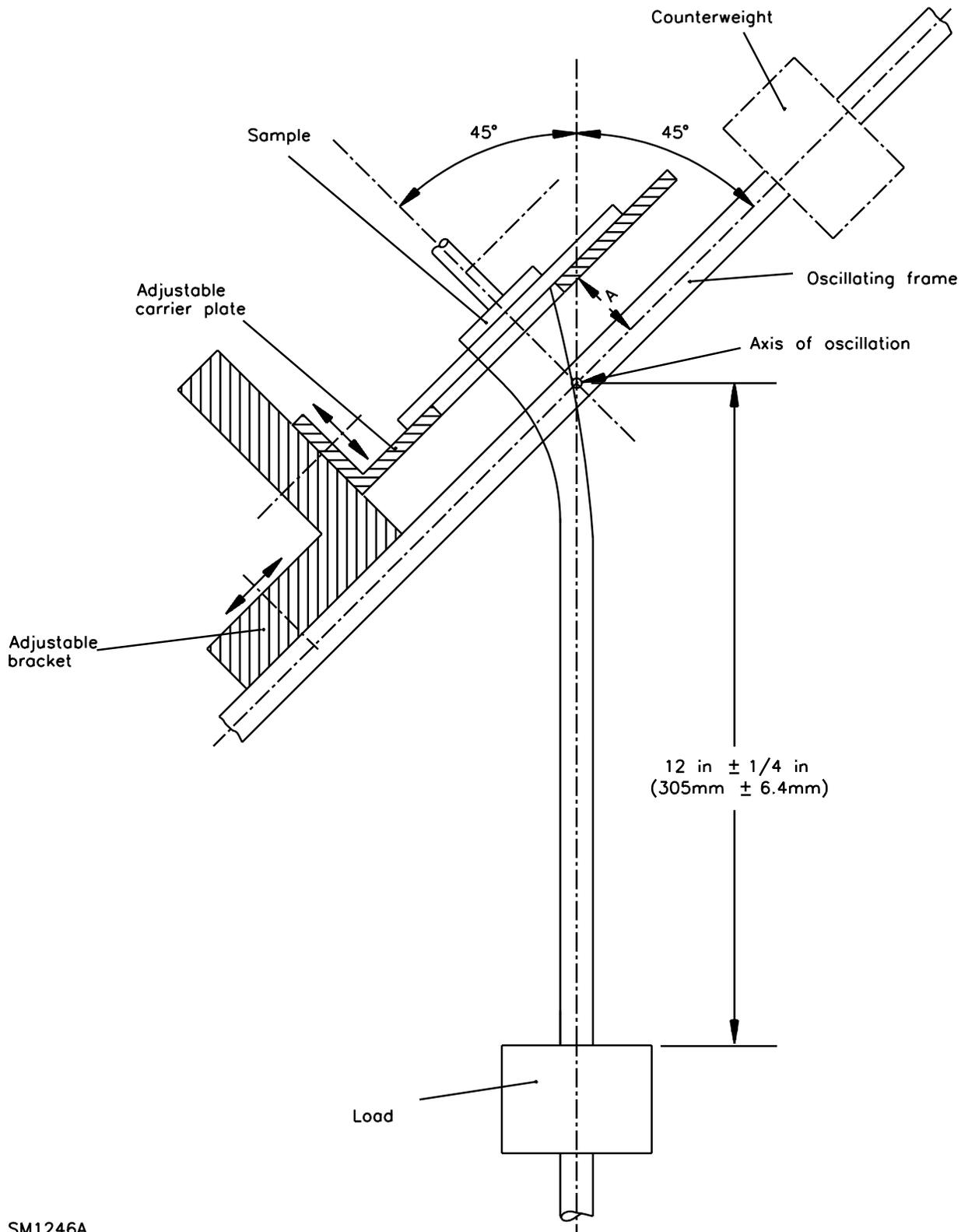
Figure 12 – Ball-pressure test apparatus
