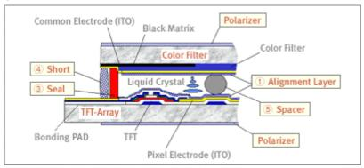
The assembly is begun by printing a polyimide alignment film on a cleaned TFT-array, and then rubbing the surface of the film with a piece of cloth wound on a roller, which orients the polyimide molecules in one direction.
