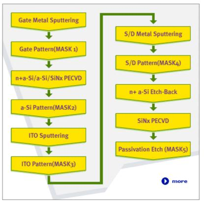
After defining the a-Si area by using photolithography and plasma dry etching, an ITO layer is deposited with a thickness of about 500A via sputtering.
