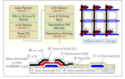
After constructing gate and storage-capacitor electrodes with 2000-3000A of a metal such as aluminum, chromium, tantalum, or tungsten, a triple layer of silicon nitride and amorphous silicon is deposited by using plasma-enhanced chemical-vapor deposition (PECVD).
