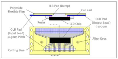
Anisotropic conducting film (ACF) is applied to the contact pads, where the stripe-shaped contact leads are formed as a group. The TCPs are then aligned and subjected to pressure-bonding.
