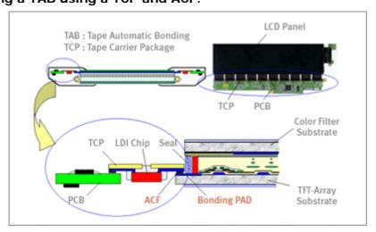
Sometimes, to minimize bezel size, the drive-circuit unit is set to the back side of the LCD module by using bent TCPs.
