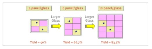
This process requires that the size of the glass substrate be steadily increased so that the number of LCD panels fabricated upon it can increase.
