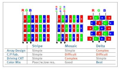
Among the many combinations of configuration and types of CF fabrication methods, the color-resist method with stripe-type RGB arrangement is currently the most popular in the CF industry.
