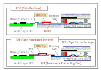
The choice of COG or TAB is determined by the peripheral area available and the limitations on bezel size for the display.
