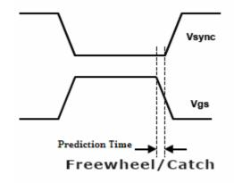
The Prediction logic uses the previous cycles to control SR operation in the present cycle. The predictive turn OFF time is adjusted by the capacitance on Pred pin. When the actual prediction time is more than that set by the capacitance on Pred pin, the IC reduces the Prediction time in the next cycle. When the actual prediction time is less than that set by the capacitance on Pred pin, the IC increases the prediction time in the next cycle.
