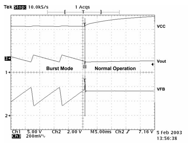
Fig. 3: Load Jump from low load to nominal load.
