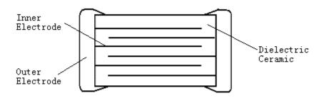
In this "multilayer" configuration, the area A is increased by virtue of many electrodes in parallel arrangement, in a construction permitting very thin dielectric thickness between opposing electrodes, such that the capacitance C is enlarged by the factor N (number of dielectric layers) and reduced dielectric thickness t', where A' is now the area of overlap of opposing electrodes.
