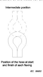
Figure 104 – Flexing positions for the hose after removal from the freezing cabinet
