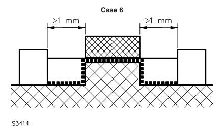
Condition: Path under consideration includes an uncemented joint with grooves equal to or more than 1 mm wide each side.
