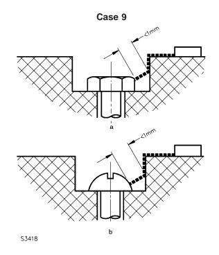
Gap between head of screw and wall of recess too narrow to be taken into account.
