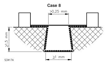
Condition: Path under consideration includes a diverging-sided groove equal to or greater than 1,5 mm deep and greater than 0,25 mm wide at the narrowest part and equal to or greater than 1 mm at the bottom.
