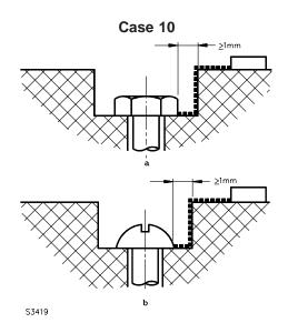
Gap between head of screw and wall of recess wide enough to be taken into account.
