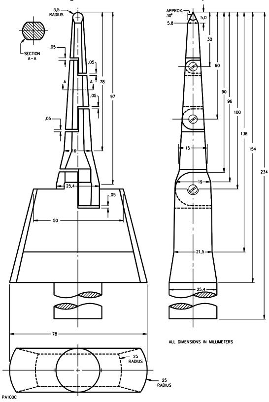
Figure 1DV – Articulate Probe with Web Stop
