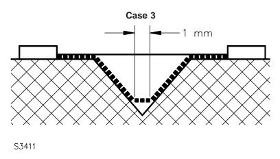
Condition: Path under consideration includes a V-shaped groove with internal angle of less than 80° and with a width greater than 1 mm.
