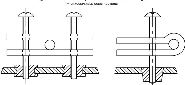
Figure 13 – Schematic representation of cord anchorages
