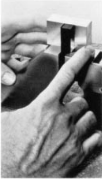
FIG. 4 Jig for Positioning Specimen for Clamping
