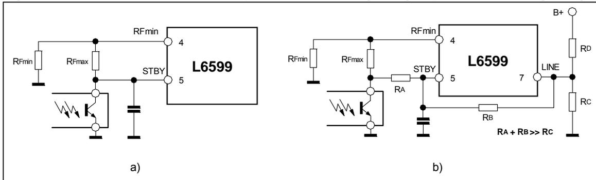
Essentially,  $RF_{max}$  will define the switching frequency  $f_{max}$  above which the L6599 will enter burst-mode operation. Once fixed  $f_{max}$ ,  $RF_{max}$  will be found from the relationship:
