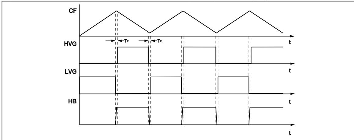
In figure 3 the timing relationship between the oscillator waveform and the gate-drive signal, as well as the swinging node of the half-bridge leg (HB) is shown. Note that the low-side gate-drive is turned on while the oscillator's triangle is ramping up and the high-side gate-drive is turned on while the triangle is
