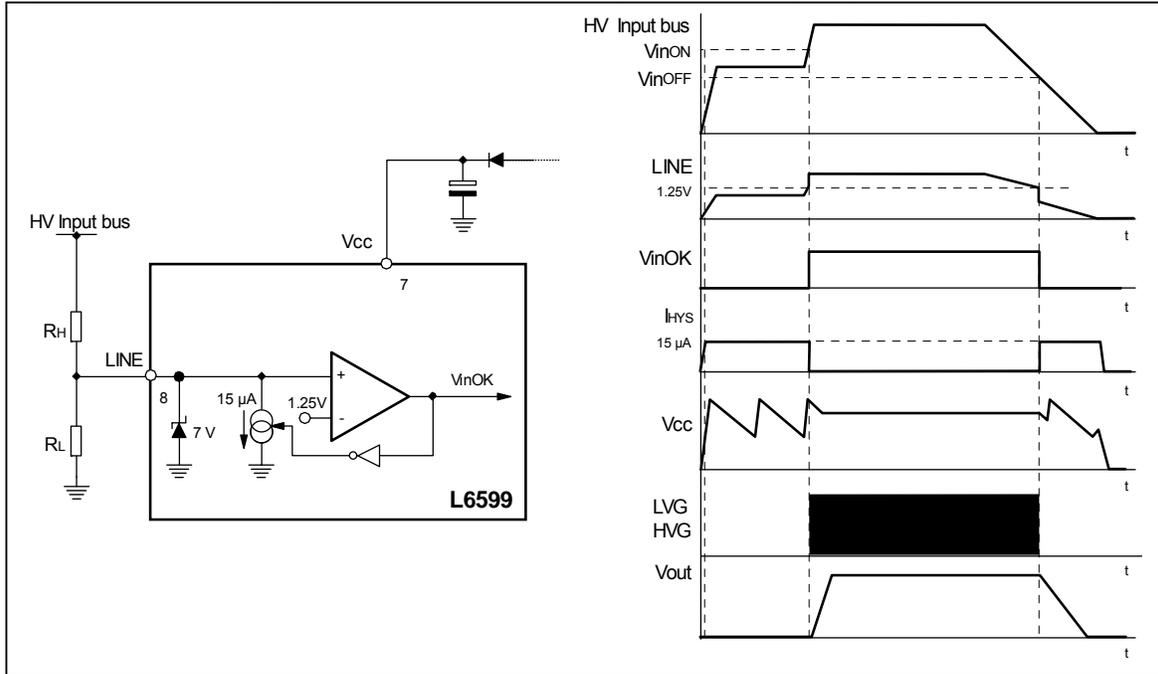
With reference to figure 10, the following relationships can be established for the ON ( $V_{inON}$ ) and OFF ( $V_{inOFF}$ ) thresholds of the input voltage:
