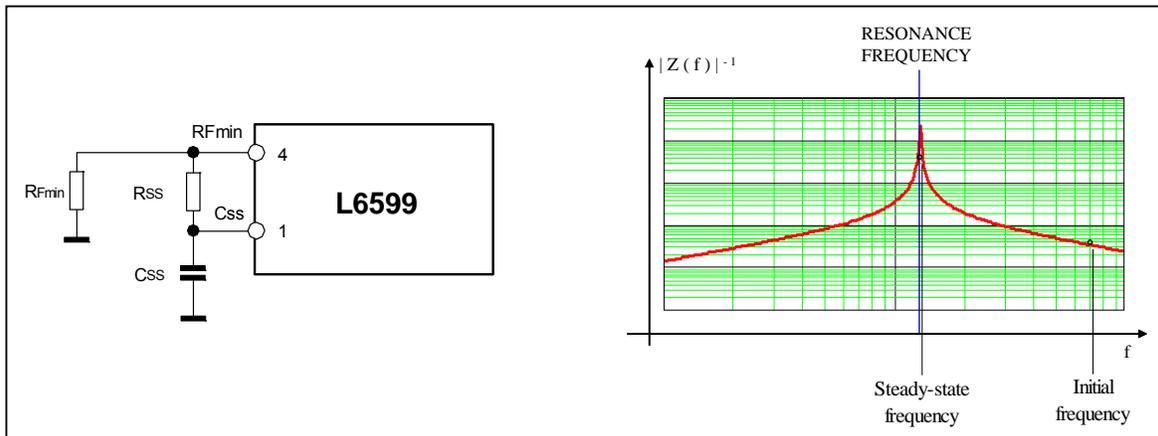
As a result, the average input current will smoothly increase, without the peaking that occurs with linear frequency sweep, and the output voltage will reach the regulated value with almost no overshoot.
