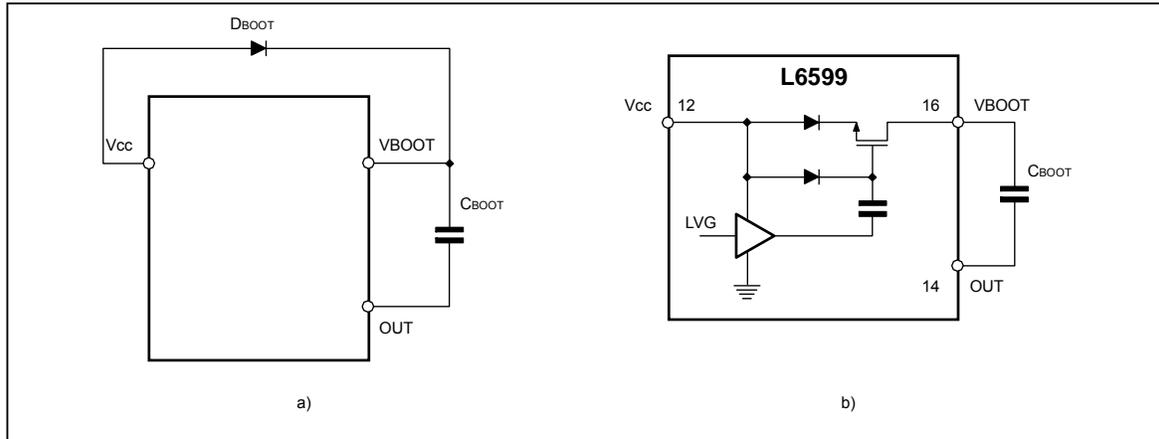
The diode prevents any current can flow from the VBOOT pin back to Vcc in case that the supply is quickly turned off when the internal capacitor of the pump is not fully discharged. To drive the synchronous DMOS it is necessary a voltage higher than the supply voltage Vcc. This voltage is obtained by means of an internal charge pump (fig. 11b).
