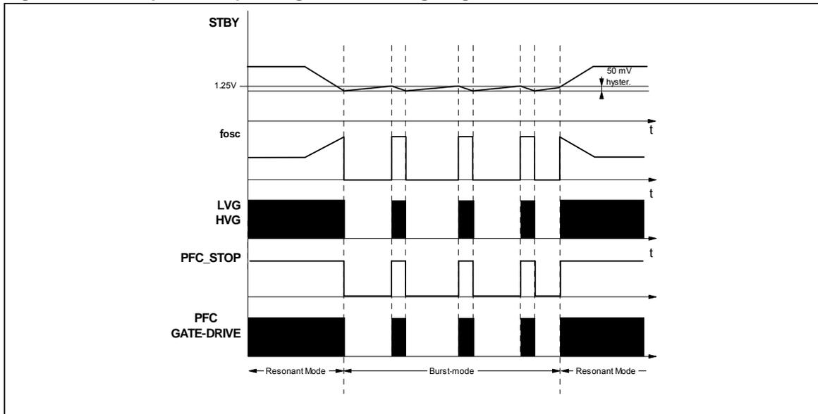
**Figure 6. How the L6599 can switch off a PFC controller at light load**
